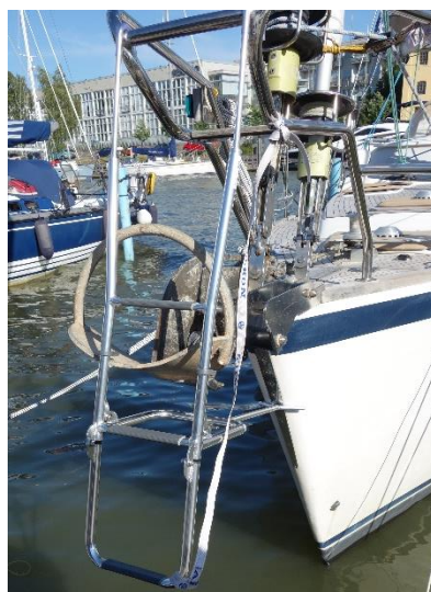
The boarding ladder
